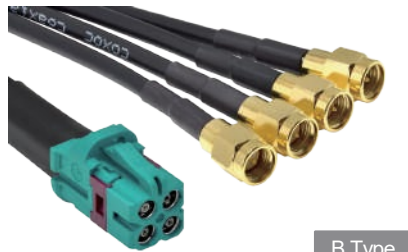
C7S8 Mini FAKRA Jack to SMA Male Plug x4 Cable Coding:A,B,C,D,E,F,Z Positions:04
