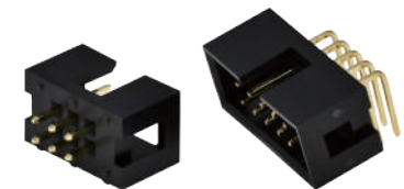
302A Box Header Pitch:2.54mm Positions:10,14,16,20,24,26,30,34,40,50,60,64
