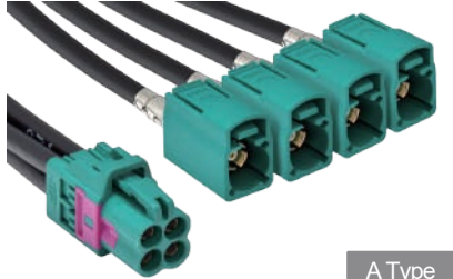
C7S5 Mini FAKRA Jack to FAKRA Jack x4 Cable Coding:A,B,C,D,E,F,Z Positions:04
